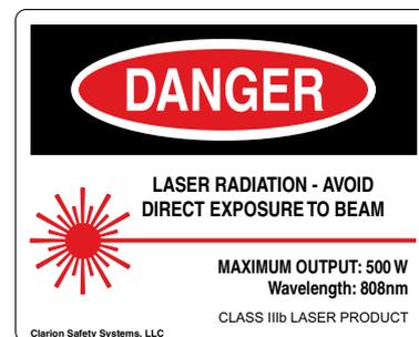
Figure 1: Examples of CDRH laser class/certification labels
